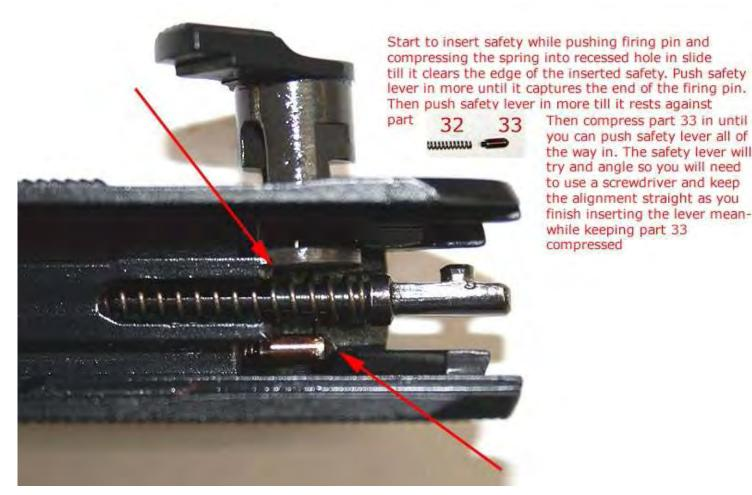
Then compress part 33 in until you can push safety lever all of the way in. The safety lever will try and angle so you will need to use a screwdriver and keep the alignment straight as you finish inserting the lever meanwhile keeping part 33 compressed
